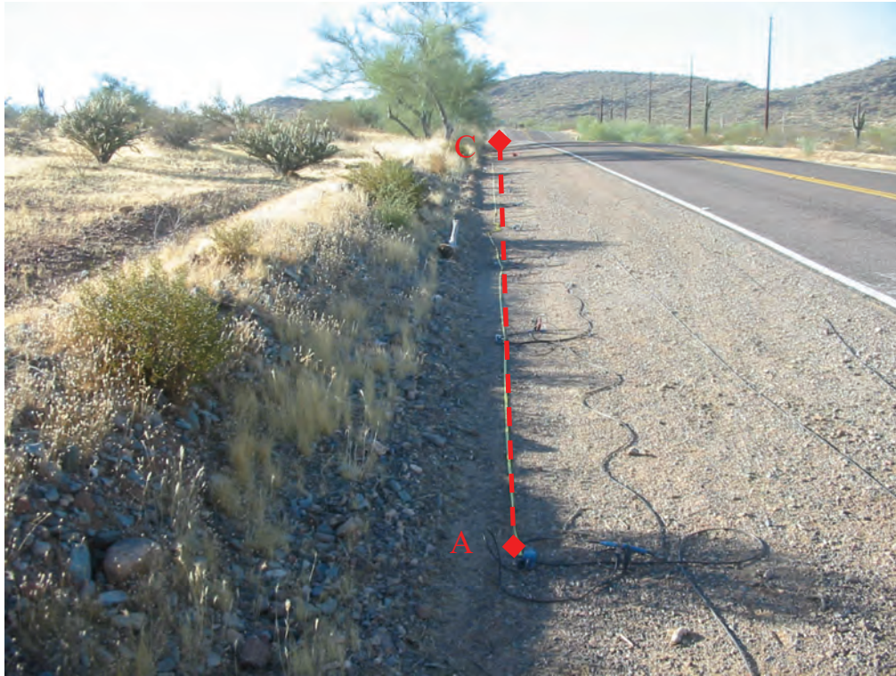
Figure 34; Photo 1: Seismic Survey Line WA-17 view looking toward the South from Shot Point A toward Shot Point C.
