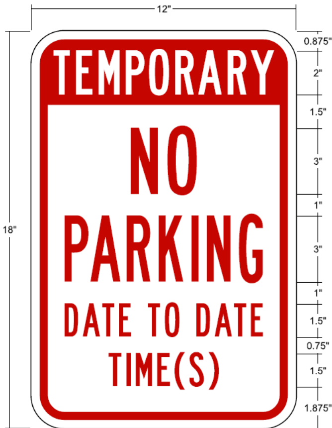
1.500" Radius, 0.375" Border, 0.375" Indent, Red on White; "TEMPORARY" B; "NO" B; "PARKING" B; "DATE TO DATE" B; "TIMES(S)" B;
