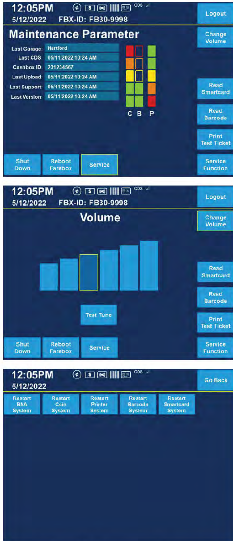
Figure 6-16 Sample Driver OCU Functions, providing convenient access to the relevant menus for the driver
