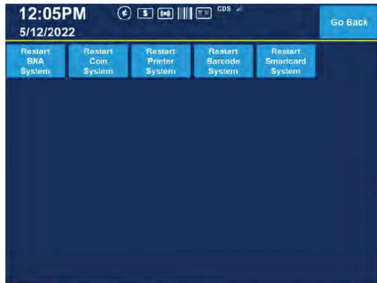
Figure 9-7 Sample Driver OCU Functions, providing convenient access to the relevant menus for the driver
