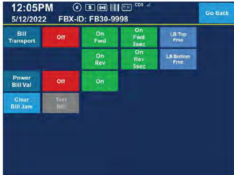
Figure 9-5 Figure 39 – Sample Bill Validator Maintenance Screen
