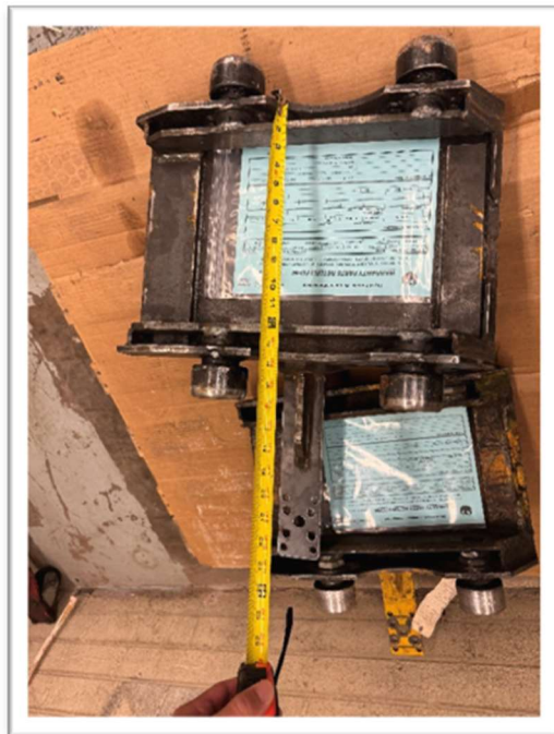
Figure 9 (Bottom) Clamp body cart with horizontal measurement (Roughly 22.5 in)
