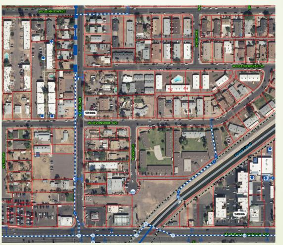
Additional work involves reconstructing curbs, gutters, sidewalks, ADA ramps, and pavement. Water service lines and a fire hydrant will be relocated, and existing fences will be temporarily removed and replaced. The pavement cut areas will be refinished with a slurry seal coat.
