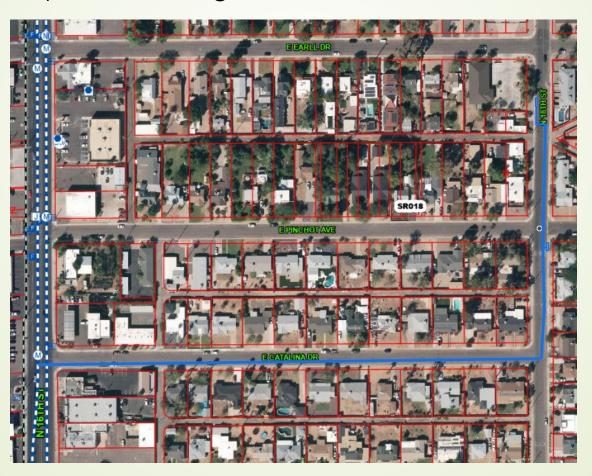
Pavement work areas will be refinished with micro-surface treatment on 16th and 18th Streets, and slurry seal treatment on Catalina Drive.
