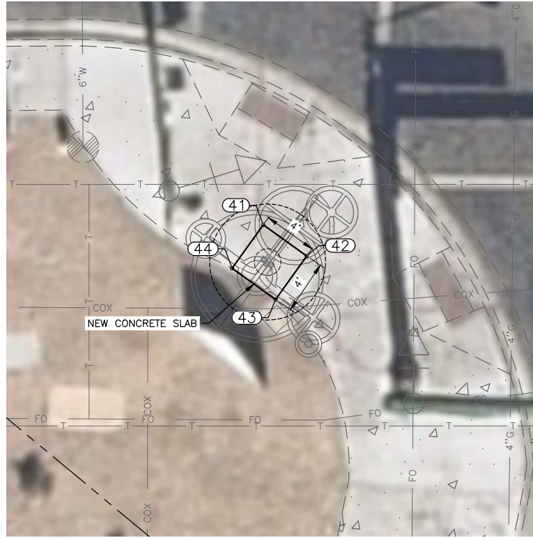
PL15 SOUTHERN AVE & 19TH AVE - SW CORNER CONCRETE PAD - HORIZONTAL CONTROL
