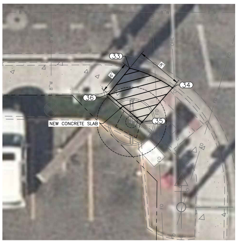
PL14 CONCRETE PAD - HORIZONTAL CONTROL
