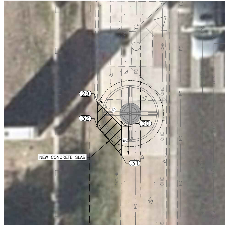
PL08 N OF MCDOWELL RD & 16TH ST - WEST SIDE CONCRETE PAD - HORIZONTAL CONTROL
