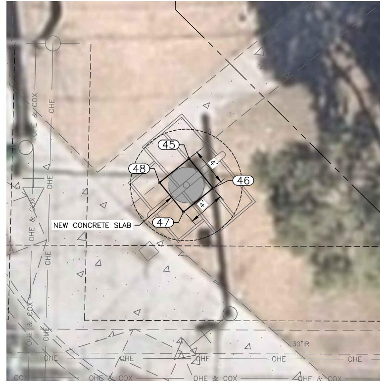
PL15 SOUTHERN AVE & 19TH AVE - NE CORNER CONCRETE PAD - HORIZONTAL CONTROL
