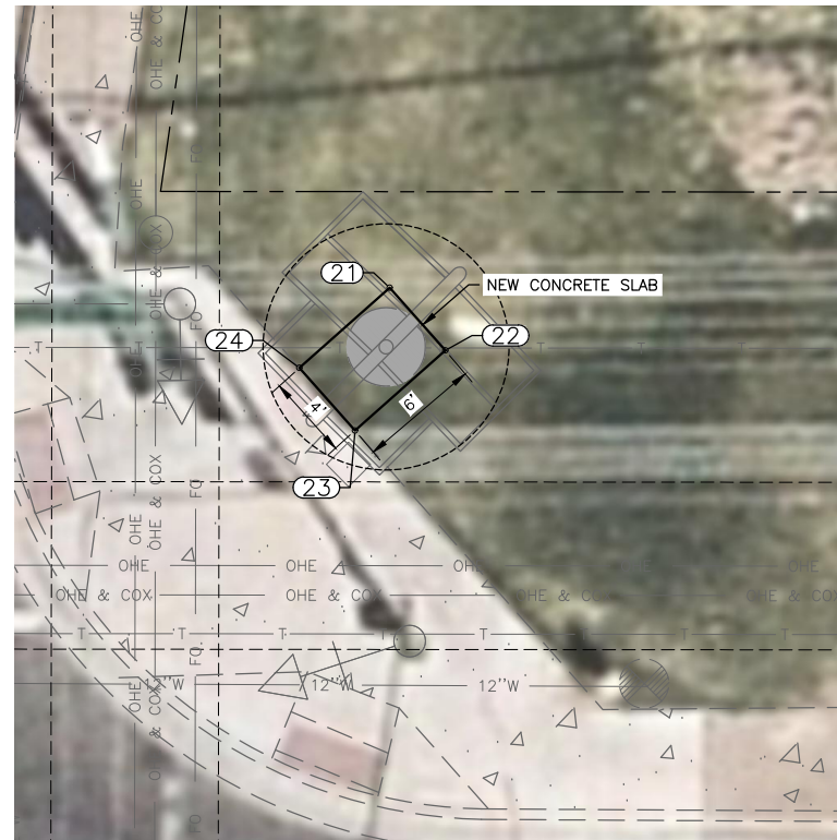
PL11 NORTHERN AVE & 35TH AVE - NE CORNER CONCRETE PAD - HORIZONTAL CONTROL
