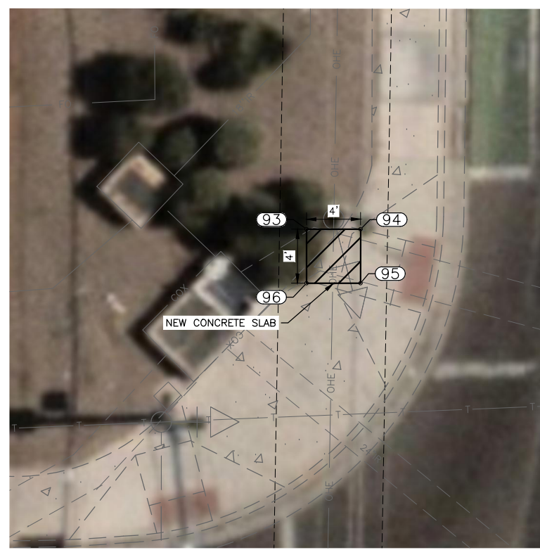
PL16 SOUTHERN AVE & 24TH ST - NW CORNER CONCRETE PAD - HORIZONTAL CONTROL
