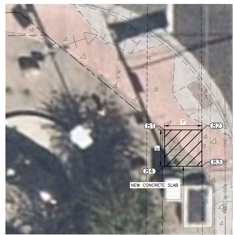
PL12 CONCRETE PAD - HORIZONTAL CONTROL
