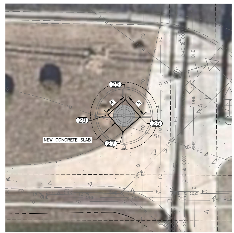
PL13 CONCRETE PAD - HORIZONTAL CONTROL
